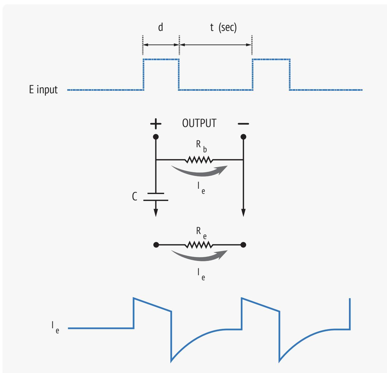
$$\frac{R_b}{R_b + R_e} = \text{Output attenuation factor due to shunt current } I_b$$
