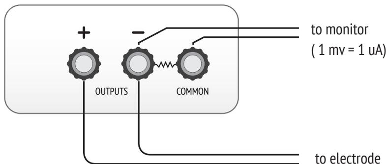
The output monitor for the constant current mode observes the voltage drop across an internal 1000 ohm shunt resistor and therefore, represents a calibration voltage of one millivolt per microamp.
